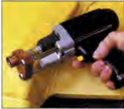
Welding gun, light and easy to handle
