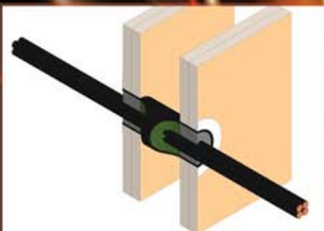
Plastic Conduit with cables FRL-/120/120
