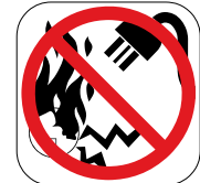
Class E Fire Electrically energised equipment
