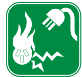
Class E Fire Electrically energised equipment
